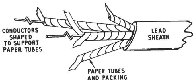
Fig. 6.14. A balanced-pair television cable
