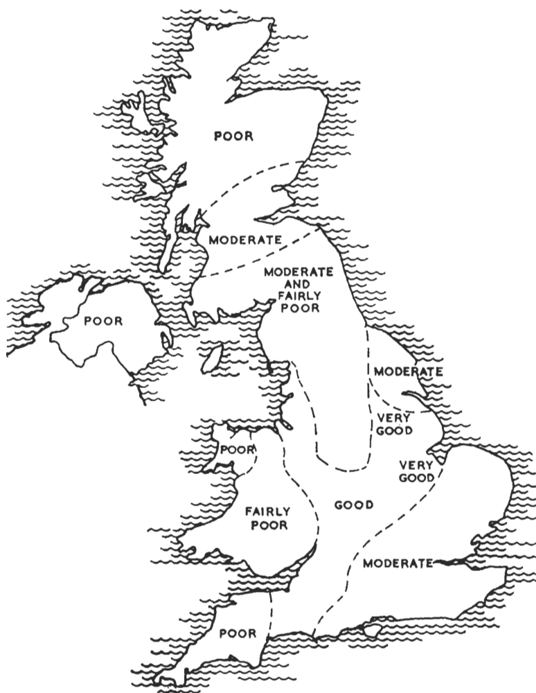
Fig. 5.45. The effect of the ground material on medium-frequency propagation over the United Kingdom
