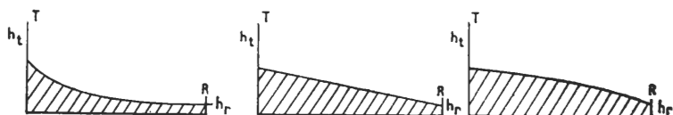
Fig. 5.52. Examples of concave, inclined plane and convex ground profiles
